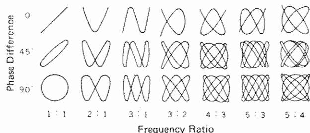
Figure 2-24. Lissajou's Figure of Different Waveforms (Frequency ratio 1 : 1)
