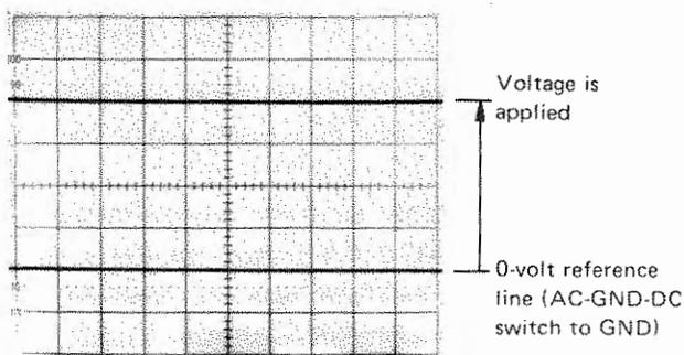
Figure 3-3. AC voltage measurement
