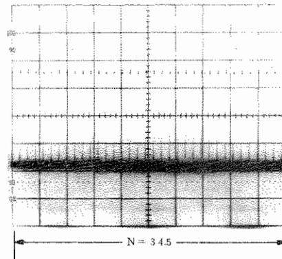
Then, 1-division graticule represents a waveform phase of  $40^\circ$  (1 cycle  $=2\pi = 360^\circ$ ). The phase difference between the two signals can be easily calculated by Equation (3-8).
