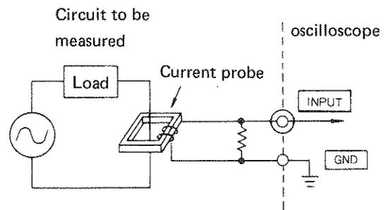
INPUTs, and its tips to both ends of the resistor inserted. Turn the VOLTS/DIV switches for CH 1 and CH 2 to the same position. The waveforms for both ends of the resistor, i. e., current waveforms, can now be observed.
