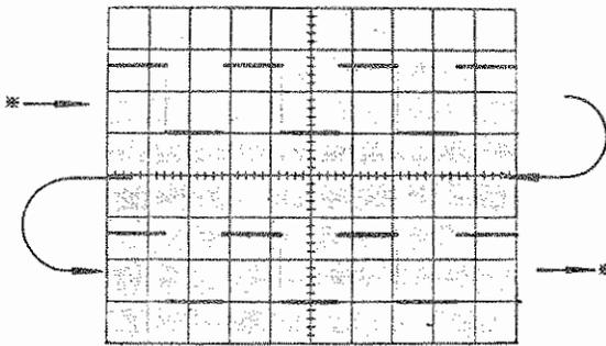
Figure 2-14. Dual-trace observation in the CHOP mode
