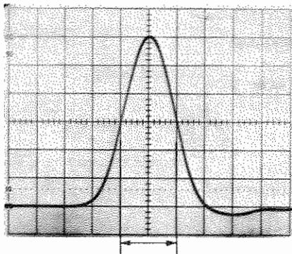
Figure 3-6. Rise (or fall) time measurement
