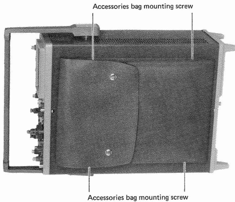
When removing the accessories bag from the upper cover of the SS-5711, remove the four accessories bag mounting screws shown in Figure 1-2.
